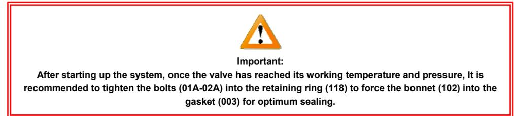
15. In case leakage is observed through the packing (004), tighten the nuts (01B-02B) carefully until the leaking stops. In case leakage through the bonnet (102) is observed, tighten the bolts (01A-02A) located in retaining ring (118).
